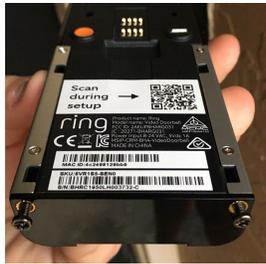
12. Align the notches from the back of the Ring doorbell to the front side of the prongs of the Ring doorbell. Once the two notches are inside each other and secure, pull down to check.
