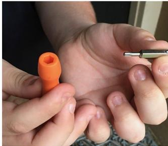
13. Take the head of the orange screwdriver and flip over, so the star head is facing upward and insert back into the orange screwdriver.
